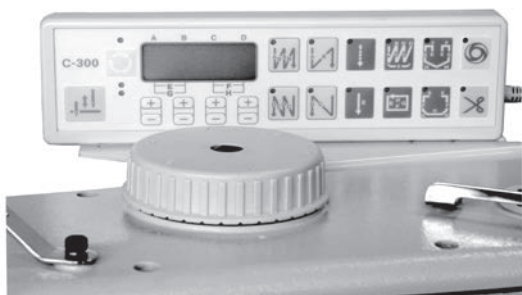
Simple setting for alternating presser foot movement
