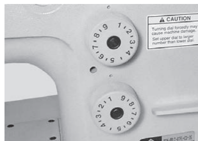
One touch switchover for two different stitch lengths (DS Device)
